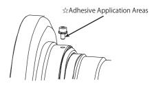
Caution: Please apply an adhesive (i.e. ThreeBond 1401 or equivalent) on thread ( $\not\propto$ ) when using it while wearing it.
